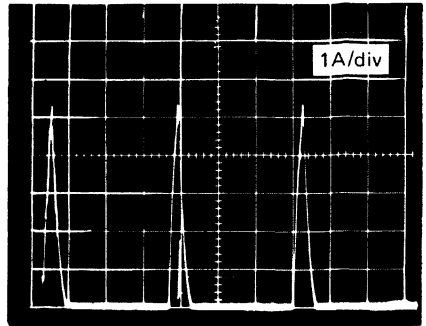
Figs 10 - Load current in short circuit conditions ( V_i = 40V , L = 300\mu H , f = 100KHz )
